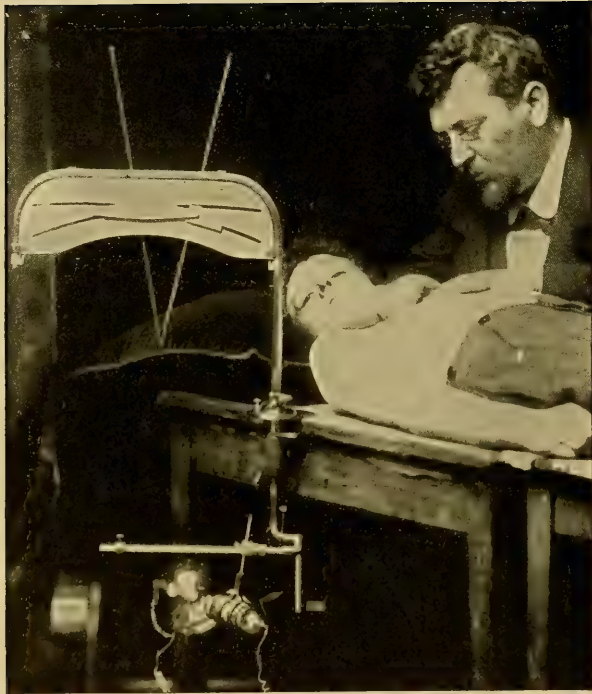
PLATE 81.—Remy Localizer. Fourth step. Now mark the two points on the skin touched by the tips of the rods. Swing the frame aside out of the way as shown in this plate. When the rods are free from the patient note the distance of the points below the frame. Then push down the rods till the points meet, and note the exact distance this is below the last position. The first measurement is the surface of the body and the last measurement is the depth of the bullet below the surface of the body in the direction shown by the two rods. The mechanical accuracy of the method is complete. During the operation the frame can be swung again into place as often as needed to verify the direction and approach to the object sought.
